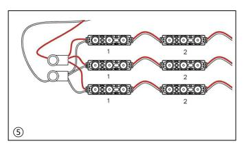
Connect LED modules to each other by connectors UY2 compliant with IP67. Note: be sure not to exceed the permitted number of LED modules in the chain.
