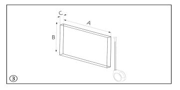
Set the right modules spacing. Consider the size of the box or channel letter mainly depth, the front face material type and desired lighting effect. If it is necessary, you can wrap the wires and dense the LED modules pitch.
