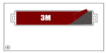
Arrange LED modules. Peel of the release paper of double-sided adhesive tapes. Then stick modules on the installing surface for preliminary mounging. Note: The adhesive tape is dor auxiliary assembly only.
