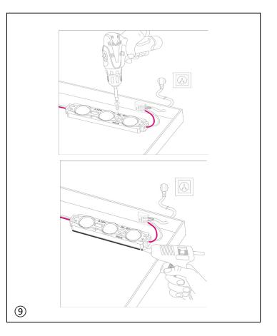
Fasten the modules and the wires permanently by screwing, riveting or the special glue. Notes: Make sure your system is unplugged.
