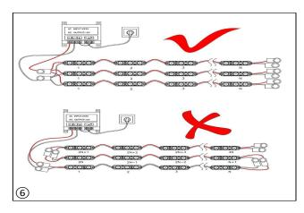
Connect the module circuitry to the proper power supply until.
